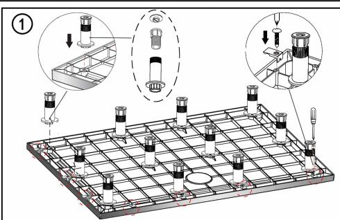
Turn the tray over and use the cardboard packaging as a protective mat, and insert the feet to the indicated positions.screw the panel clips into position on the side that the panels will be attached.
