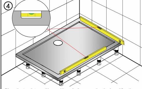
Place the tray into position and lever both ways using the legs.After the tray has been levelled adjust all the inner feet to stabilise the tray. When level fix these legs to the floor with silicon sealant.
