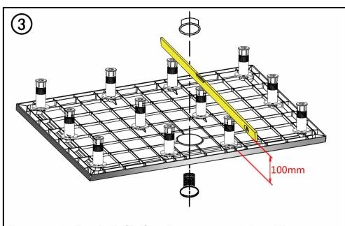
Remove protective plastic film from the areas near waste and those sides of the tray which will be against a wall. Fit the shower tray waste. all feet should be adjusted to 100mm.
