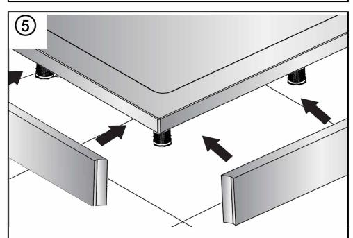
first fix the rebated panel pushing it firmly on to the panel clips,then fix the remaining panel in the same manner.
